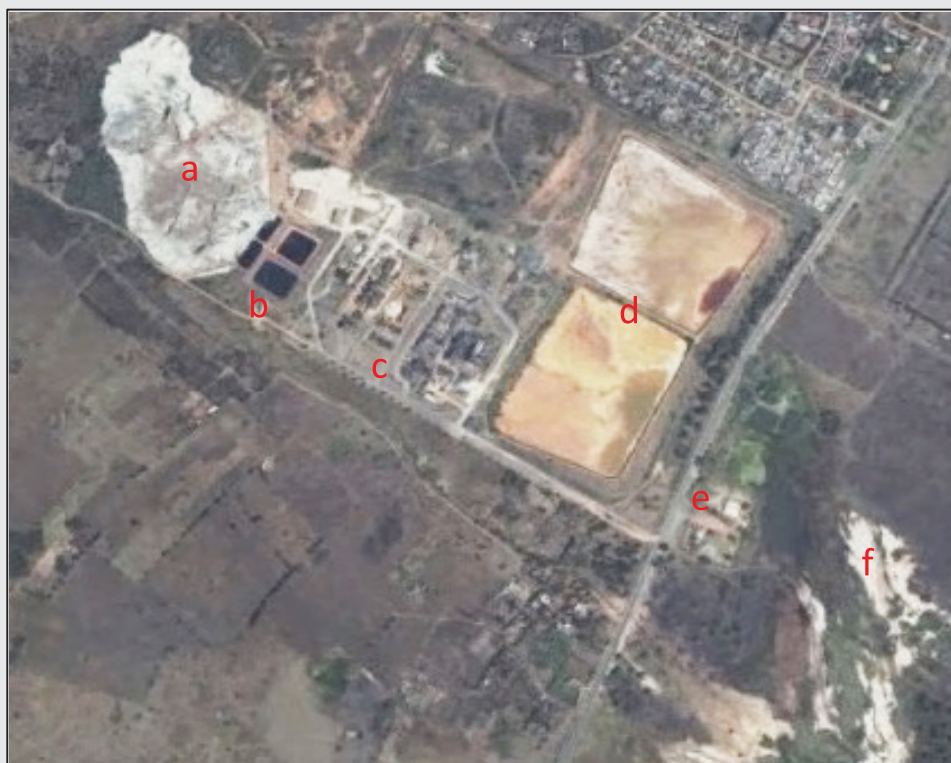
Google Earth image showing a) pyrite stockpile; b) ARD capture from stockpile; c) bioleaching and water treatment plant area; d) new contained tailings; e) water control pond; f) old (pre-KCCL) impacts from acidic water discharge.
